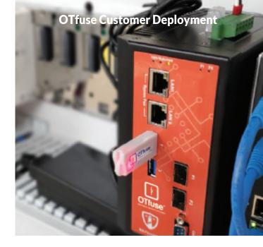
Once switched into 'Protection' mode, the OTfuse will apply its customized policy to the Endpoint Segment assets directly and in real time, while alerting the customer via their existing SCADA system of any blocked events. Customers can interact with a single OTfuse directly from their control room, or make use of a centralized web-based management console for batch review of policies and events across a large number of individual appliances.
